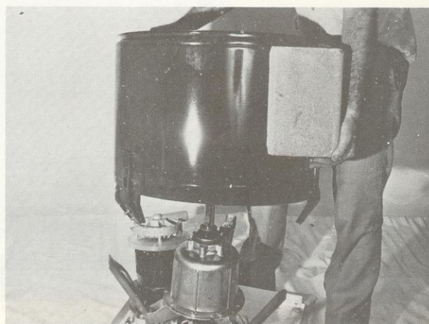
37- Remova o tanque.
