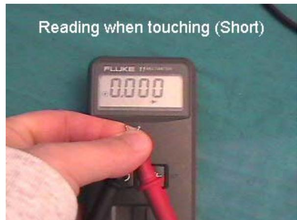
To test the power cord take one lead and attach it to one prong that plugs into the wall and the other lead into one of the holes that plug into the PS2. You should get a low reading just like you did when you tested above. If not, move to the other hole. Do that for each hole and prong to check both wires inside the cable. If both check good then you are ready for the next step. If not, then you have a bad cord and it will need to be replaced.
