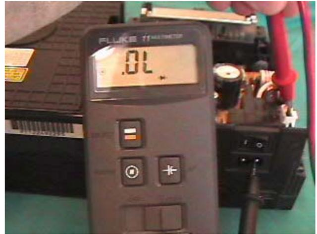
Last we will check the fuses. There are two located on the power supply board. (see photo)
