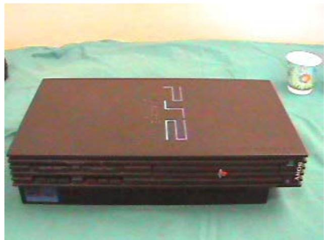
Pull up on the cover from the back and work it free and lift about 1/2 inch. Move the shell forward a little, sideways, so that the **Eject/Reset buttons** are **not blocking** the shell and the CD tray comes clear, and it can be lifted off. Just play around with it a little and you should get it.
