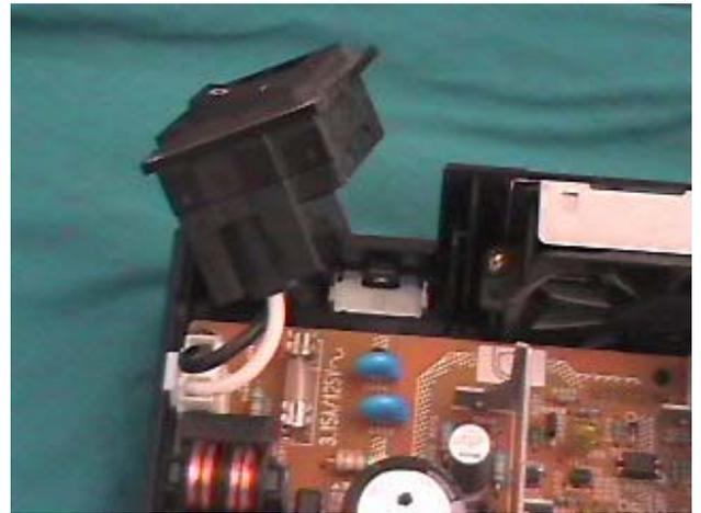
When you get your replacement board, just take out the 4 screws on the corners holding it in and pull up on it to remove it from the 4 pin connector (see photo). You will also need to slide the power switch assembly out of your way. Unplug the white 2 wire connector from the power supply board and slide the assembly out of the slot it fits in on the case. (see photo)
