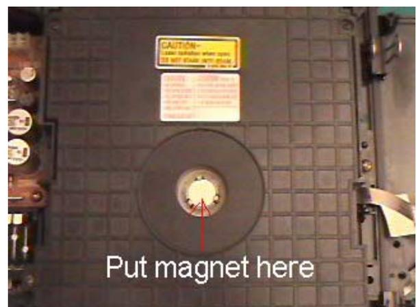
**NOTE:** Here is a picture of the one I just did with the sheet magnets in place. It's up to you at this point if you want to continue. This may be all that is needed to fix your problem. Put the cover back on and try it out. If it doesn't work you will need to take the cover back off and then continue with the next step, or you can continue now. The choice is yours.
