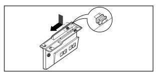
4. Pull forward the insulating material of the cooling cycle unit and remove the wire terminal and insulating material.
