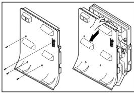
5. Remove 2 screws securing refrigerator duct and pull it out by following the arrow.
