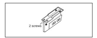
3. Pull out the holder of the cooling cycle unit and disconnect wire terminals.
