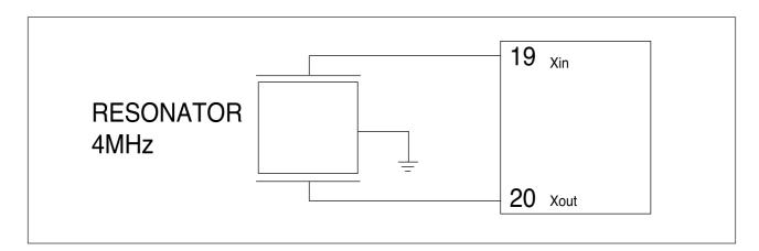
◆The role of this circuit is generation of synchronous CLOCK for transmission/reception of informations of the logical elements inside MICOM and the basic time for the calculation of time. Rated parts must be used in the division of RESONATOR because the calculation time of MICOM is changed or cannot work if specification is changed.
