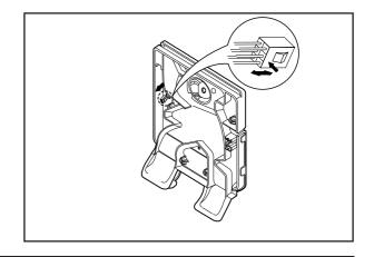
6. Remove 3 screws from the back cover of the cooling cycle unit and remove the latch with (+) driver.
