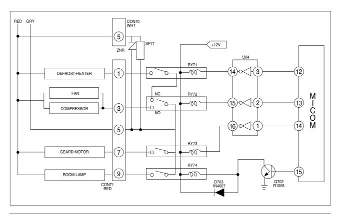
◆ If at MICOM PORT begins to output "High" signal which corresponds to electrical load which we intend to work, DRIVER IC(KA2657) is turned ON and at this moment, corresponding electrical load starts to operate because the DC12 yield the electric current which flows corresponding RELAY COIL and RELAY contacting point is set to be ON so corresponding electrical load begins to operate.
